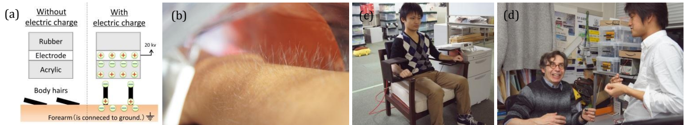
Figure 1. (a) Principle of a prototype device, (b) Forearm hair behavior with electrostatic force, (c) Schematic view of the Chilly Chair, (d) Surprised expression on a participant when both audio stimulation and piloerection were presented.
