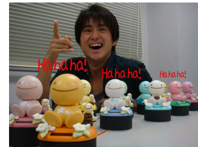
Figure 1 System overview. The dolls play laughter sounds and shake their heads in synchronism with the user’s laughter.
